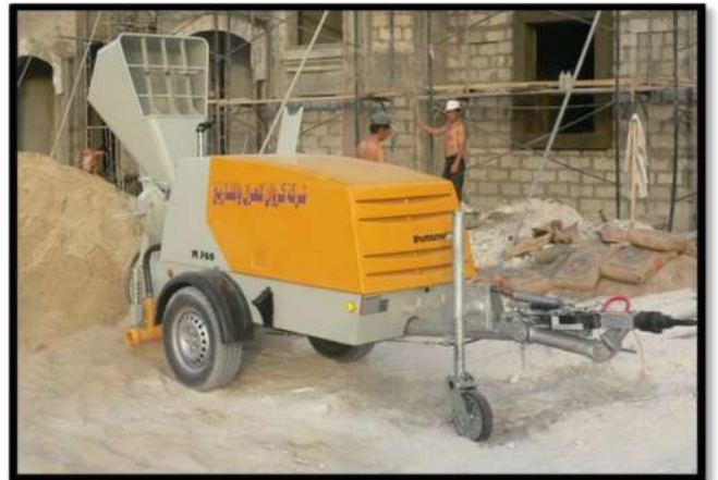
CONCRETE PUMP PUTZMEISTER M760
